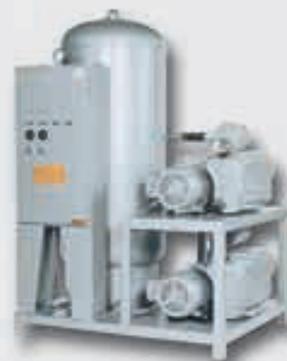
Duplex expandable model uses a common skid for mounting vacuum pumps, electrical controls, and a vertical receiver.
